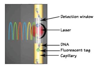
Each fluorescent dye emits its maximum fluorescence at a different wavelength. The emitted fluorescence is passed through a diffraction grating and is captured by a CCD (charge-coupled device) camera. The grating separates the fluorescence of each dye, although there is a degree of overlap. The output is sufficiently separated to allow for the analysis of loci which are of similar size but have different fluorescence labels.
