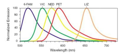
The precise spectral overlap between the dyes is measured by running DNA fragments labeled with each of the dyes in separate CE injections, producing a matrix file. The matrix file allows for multi-component analysis. The appropriate matrix file can be applied to data on a CE run, and the software automatically applies a mathematical matrix calculation (using the matrix file) to all sample data to adjust for the spectral overlap.
